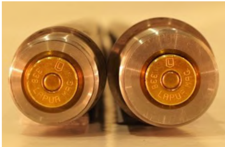
Larger stronger barrel tenon for higher pressure
